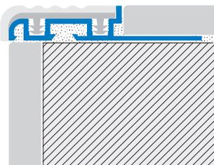
**STAIRTEC FSF-A\* Aluminium + Synthetic insert width 30 mm**
